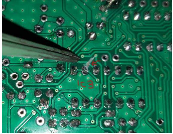
Solder in Bridge between outer Pins of Q6 Pads. Place 10nF Capacitor into outer Pins of PCB Q4, Place Resitor 10K from Middle Pin of Q4 to Outer Pin of Q4 (BNC-Jack Side of PCB)
