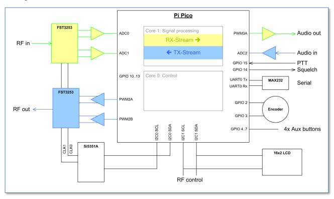
Note that the ADCs and DACs have a maximum range of 3V3.
