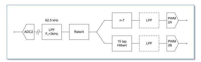
The TX stream is the inverse of the RX stream: the same components can be found here as in the RX stream. As in the RX the SSB is generated by converting the I-samples into Q-samples through a 15 tap Hilbert transform. The Q output is multiplied by -1 for USB and +1 for LSB, the I-samples need to be delayed by 7.
