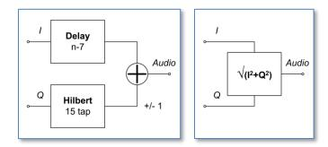
For SSB demodulation, the decimated I and Q samples are stored in a 15-sample delay line. A 15-tap Hilbert transform on the Q channel is done and the result is subtracted from or added to the n-7 sample in the I delay line to obtain the USB or LSB audio output respectively.
