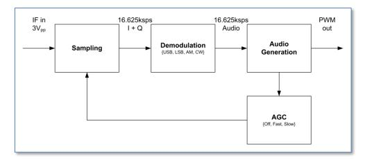
The RX stream can be functionally segmented into a part that does the sampling and decimation, a part that does the actual demodulation type of choice, and a part that does the audio generation. The output gives rise to an AGC feedback, where the amplification of the input is changed in factors of 2. The AGC mechanism is only local, the RX frontend optionally includes larger scale attenuation of pre-amplification of the received signal.
