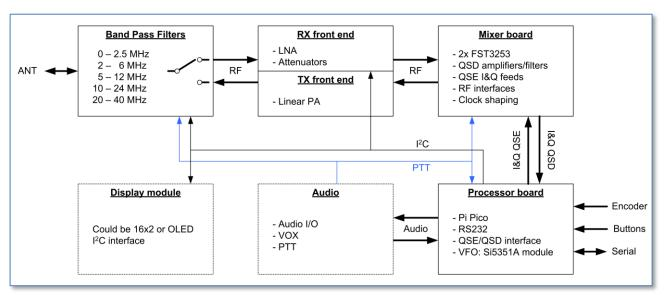
The signal path leads from Audio board to BPF and vice versa. Internal control is done through an I<sup>2</sup>C bus and a discrete PTT signal. The latter is either passed through from a microphone, generated by the VOX or issued by SW in the Processor.
