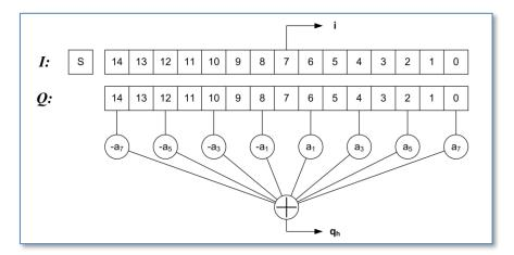
The Q delay line array has a length of 15, to enable a 15-tap classic Hilbert transform. The even samples have a zero coefficient so, as in the above figure, only 8 of the samples are used in the calculation. Due to symmetry of this classic Hilbert transform only 4 multiplications have to be performed. The resulting transformed output is in phase with the  $8^{th}$  sample in the array, being I[7], Q[7] and the calculated  $Q_h$ .
