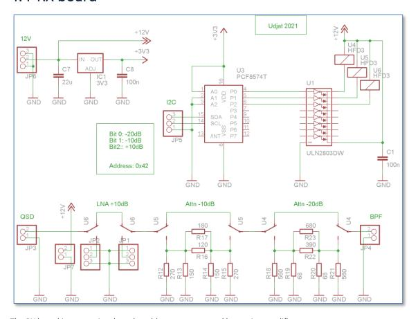
The RX board just contains the selectable attenuators and low noise amplifier.
