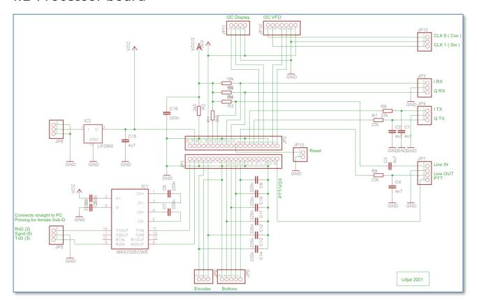
The processor board hosts the Pico module, the Si5351A VFO module and the user interfaces. There is also a serial interface that provides a monitor with a command line interface. The audio handling and PTT/VOX circuitry is moved outside the CPU/IO board, for modularity reasons.
