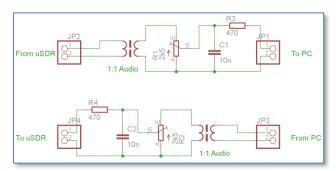
The second circuit is used in the cable that connects PC with uSDR-Pico, and serves as galvanic separation; PCs can be rather noisy... The trimmers can be used to adjust the required levels.
