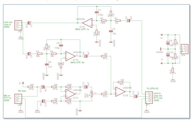
The first is buffering and pre-amplifying the line and microphone channels, as well as an additional 3kHz low pass filter. The line in signal is amplified 6dB to get some extra range for level optimization. The signal that goes to the ADC should be close to  $3V_{pp}$ . The mike signal is more or less balanced and amplified 10dB. In the current version this is still to be tested. The mike PTT signal is only enabled when No VOX is selected, otherwise the PTT is level controlled.
