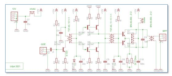
The TX board contains a wideband linear driver as proposed by Harry Lytthal (SMOVPO) that outputs up to 500mW. The end-stage, also a class AB push-pull configuration, should be good for about 5 Watts. The symmetry of this circuit should better suppress the even harmonics.
