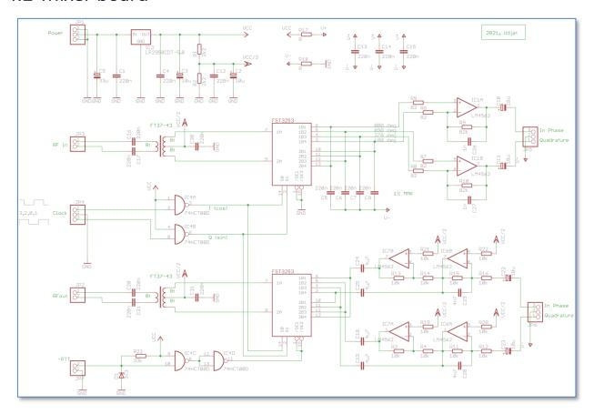
The mixer board hosts the two mixers, QSD for RX branch and a QSE for the TX branch. The switches are clocked from the Si5351 board, through two HCT NAND gates that take care of level shifting and some signal cleanup. TX path can be disabled when PTT is not active. RX path is always enabled.
