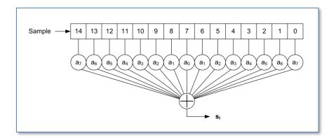
Several 15-tap low pass filters have been created, with a corner frequency of  $F_c$ =3kHz. The stop-band depends on the actual sample rate the filter is designed for. It usually starts around 5kHz, with a level of -40dB or better. The code contains filters for 62.5 kHz, 31.25 kHz and 15.625 kHz sample rates, although only first and last are actually used.
