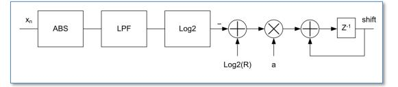
The process determines signal level by taking its absolute value and then leading it through an exponential averaging (low-pass) filter:
