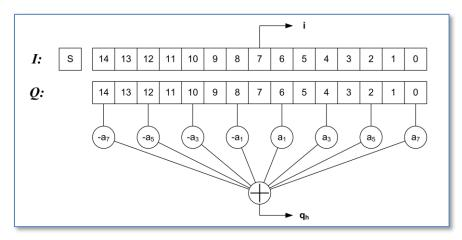
The Q delay line array has a length of 15, to enable a 15-tap classic Hilbert transform. The even samples have a zero coefficient so, as in the above figure, only 8 of the samples are used in the calculation. Due to symmetry of this classic Hilbert transform only 4 multiplications have to be performed. The resulting transformed output is in phase with the  $8^{th}$  sample in the array, being I[7], Q[7] and the calculated  $Q_h$ .
