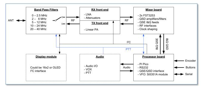
The signal path leads from Audio board to BPF and vice versa. Internal control is done through an I<sup>2</sup>C bus and a discrete PTT signal. The latter is either passed through from a microphone, generated by the VOX or issued by SW in the Processor.
