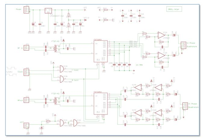
The mixer board hosts the two mixers, QSD for RX branch and a QSE for the TX branch. The switches are clocked from the Si5351 board, through two HCT NAND gates that take care of level shifting and some signal cleanup. TX path can be disabled when PTT is not active. RX path is always enabled.
