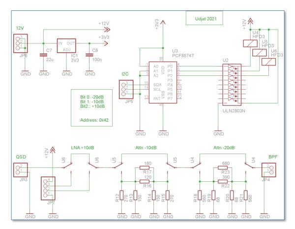
The RX board just contains the selectable attenuators and low noise amplifier. Both boards have the same form factor as the CPU and Mixer, i.e. 51mm x 81mm (2.0"x3.2")
