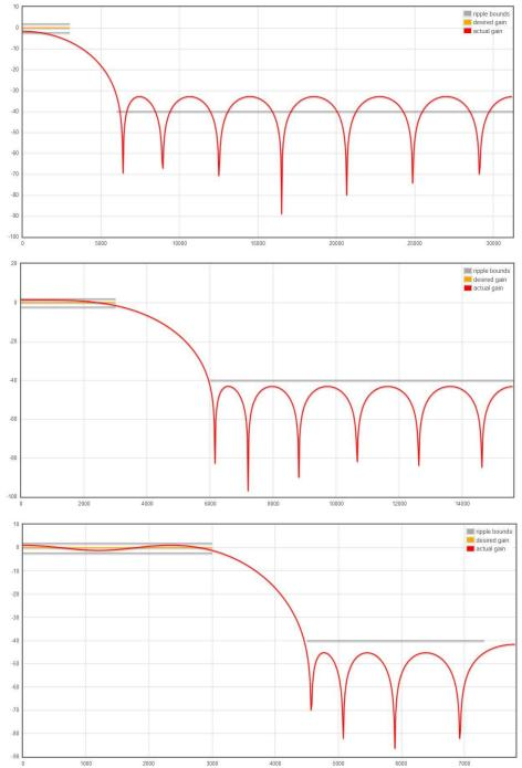
T-filter parameters 62500, 31250 and 15625 sample rates, passband 3kHz ripple <5dB, stopband from 6kHz at -40dB:
