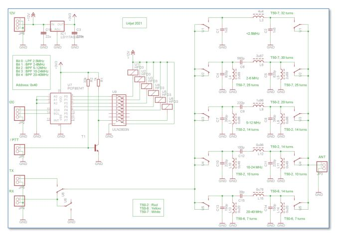
The 5 band filters are selected through relays, controlled from the Pico via the  $I^2C$  bus. A sixth relay is connected to the PTT signal, and connects either RX or TX path to the filters.
