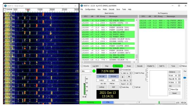
As the screendump shows, the current version works nicely on the 40m FT8 channel. The AGC now also works, albeit not yet controllable from the menu. It makes sure that the output signal is maintained between  $1.6V_{pp}$  and  $3.3V_{pp}$ .
