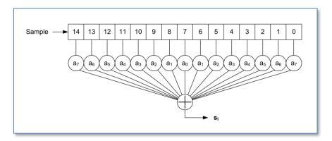
Several 15-tap low pass filters have been created, with a corner frequency of  $F_c$ =3kHz. The stop-band depends on the actual sample rate the filter is designed for. It usually starts around 5kHz, with a level of -40dB or better. The code contains filters for 62.5 kHz, 31.25 kHz and 15.625 kHz sample rates.
