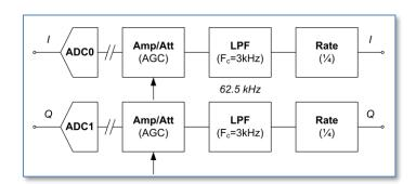
The RX stream function is called every 16usec, where the most recent I and Q samples are taken from the buffer, resulting in 62.5kHz sampling rate for each channel.
