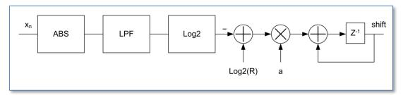
The process determines signal level by taking its absolute value and then leading it through an exponential averaging (low-pass) filter:
