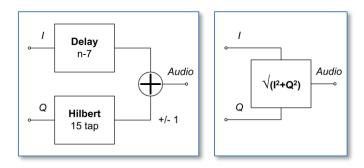
For SSB demodulation, the decimated I and Q samples are stored in a 15-sample delay line. A 15-tap Hilbert transform on the Q channel is done and the result is subtracted from or added to the n-7 sample in the I delay line to obtain the USB or LSB audio output respectively.
