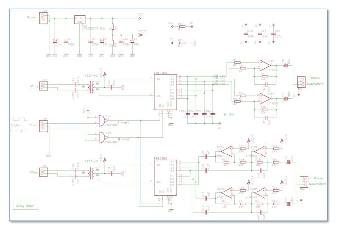
The mixer board hosts the two mixers, QSD for RX branch and a QSE for the TX branch. The switches are clocked from the Si5351 board, through two HCT NAND gates that take care of level shifting and some signal cleanup.
