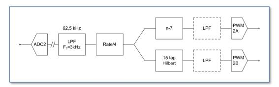
The TX stream is the inverse of the RX stream: the same components can be found here as in the RX stream.
