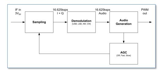
The RX stream can be functionally segmented into a part that does the sampling and decimation, a part that does the actual demodulation type of choice, and a part that does the audio generation. The output gives rise to an AGC feedback, where the amplification of the input is changed in factors of 2. The AGC mechanism is only local, the RX frontend optionally includes larger scale attenuation of pre-amplification of the received signal.
