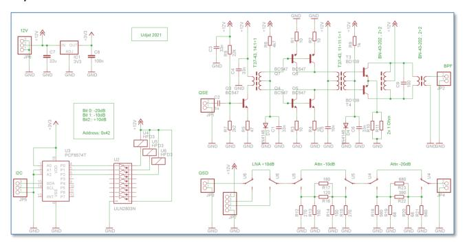
The RX/TX board provides a TX power amplifier and an RX selectable amplifier/attenuator in independent paths. The RX/TX switching is allocated to the BPF board.
