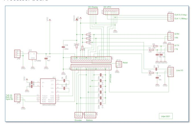
The processor board hosts the Pico module, the Si5351A VFO module and the user interfaces. There is also a serial interface that provides a monitor with a command line interface. The audio handling and PTT/VOX circuitry is moved outside the CPU/IO board, for modularity reasons.
