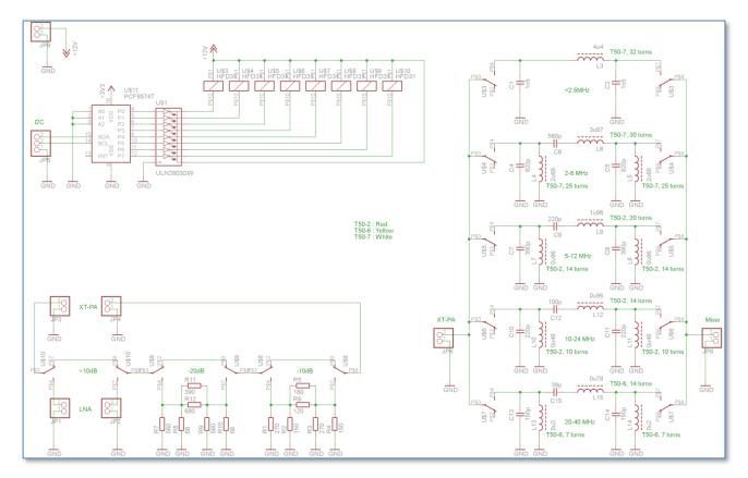
The 5 band filters and the attenuators/LNA are selected through relays, controlled from the Pico via the  $I^2C$  bus. The (roughly octave) filters are calculated with ELSIE, and have the following pass-through characteristics:
