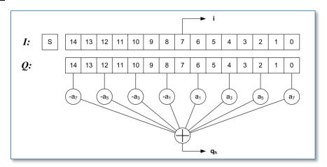
The Q delay line array has a length of 15, to enable a 15-tap classic Hilbert transform. The even samples have a zero coefficient so, as in the above figure, only 8 of the samples are used in the calculation. Due to symmetry of this classic Hilbert transform only 4 multiplications have to be performed. The resulting transformed output is in phase with the 8<sup>th</sup> sample in the array, being I[7], Q[7] and the calculated  $Q_h$ .
