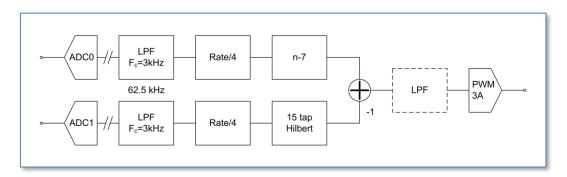
The RX stream function is called every 16usec, where the most recent I and Q samples are taken from the buffer, resulting in 62.5kHz sampling rate for each channel.
