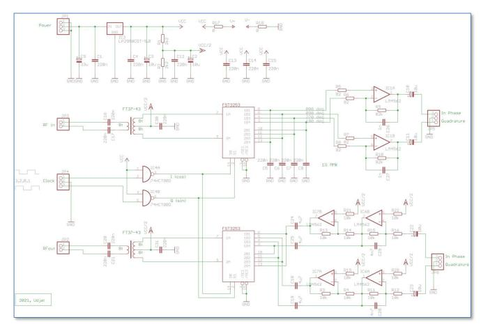
The mixer board hosts the two mixers, QSD for RX branch and a QSE for the TX branch. The switches are clocked from the Si5351 board, through two NAND gates that take care of level shifting and some signal cleanup.
