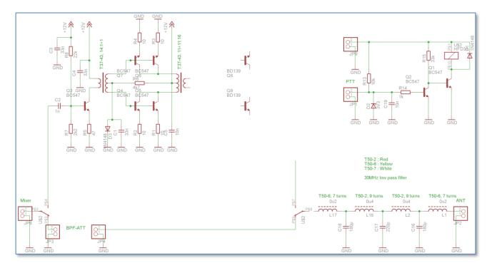
The transmitter PA board is still highly under development. The idea is to have a wideband linear driver as designed by Harry Lytthal (SMOVPO) that outputs up to 500mW. The end-stage should be good for a few Watts, but needs to be tried out.
