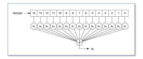
Several 15-tap low pass filters have been created, with a corner frequency of  $F_c$ =3kHz. The stop-band depends on the actual sample rate the filter is designed for. It usually starts around 5kHz, with a level of -40dB or better. There are filters for 62.5 kHz, 31.25 kHz and 15.625 kHz sample rates.
