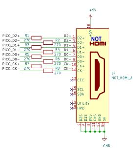
The raspberry end of a RPi Pico is surface mounted onto this board, to fit a DMI (the H is silent) connector onto the end opposite the micro-USB. It's pretty low-profile on the bottom, so you can fit headers to the remaining Pico I/O pins and stick the board into a breadboard. Micro-USB one end, video the other end. **Luke Wren**
