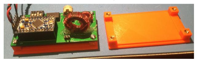
Figure 5: Board and sub-plate.
