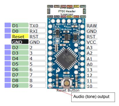
Figure 4: Audio output from Pro Mini.
