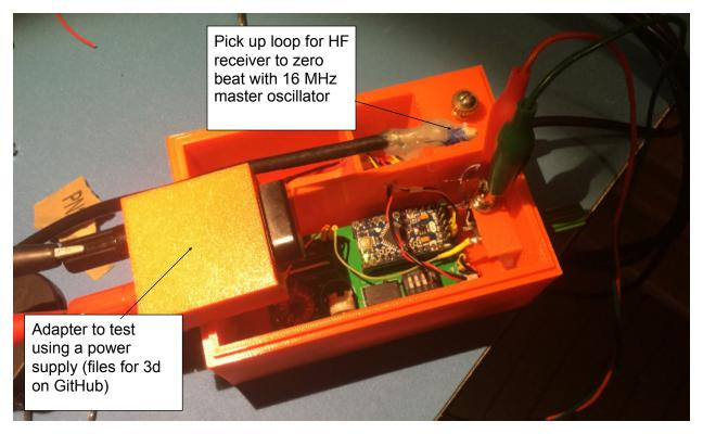
Figure 7: Receiver calibration method.
