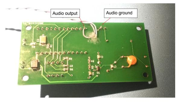
Figure 3: Bottom of board showing connections for audio output.
