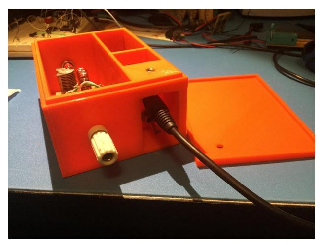
Here the sync cable is plugged in. Plan to make a 3D cover to slide in and cover the recessed on/off switch and sync compartment
