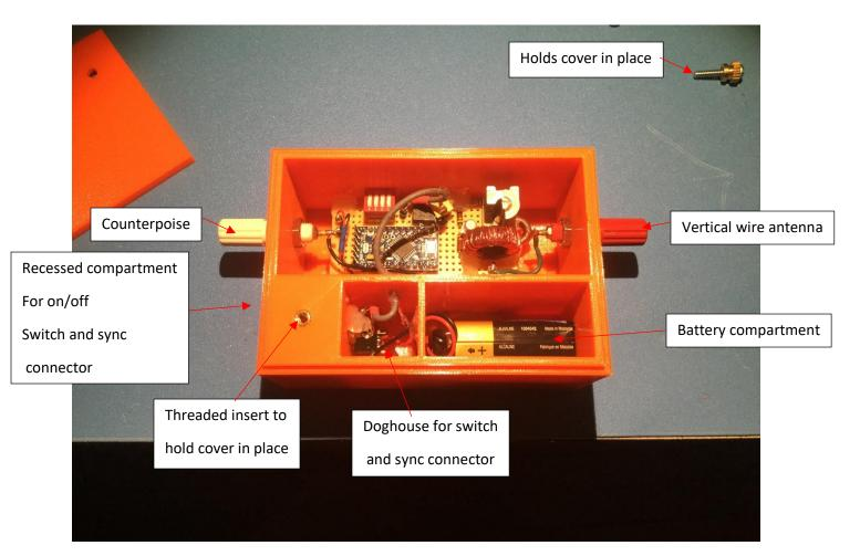
The 80 meter practice micro fox box is generic so that a larger electronics assembly can be housed. Plan to re-use the case for the VHF CW practice micro fox.
