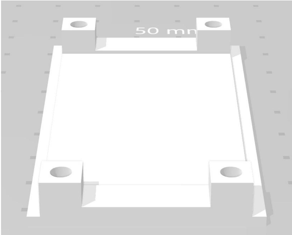
*Figure 10: The sub-base for mounting the PCB.*
