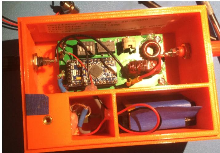
Figure 14: Battery installed.
